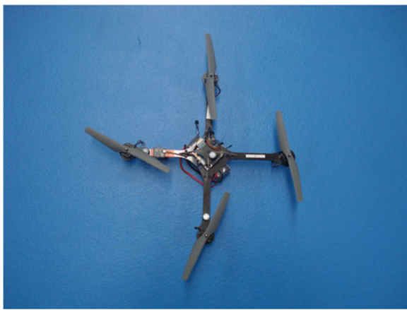
Fig. 8 Hummingbird quadrotor from Ascending technologies used in the experiments
