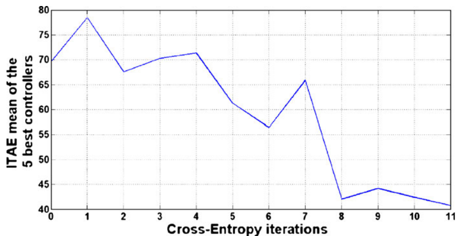
Fig. 12 Evolution of the ITAE error during the 12 Cross-Entropy iterations. The ITAE value of each iteration correspond to the mean of the first 5 of 30 controllers of each iteration
