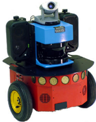
Fig. 10 The experimental setup at the Distributed Intelligence Laboratory of University of Tennessee. Left: a Pioneer-3DX mobile robot. Right: the team used in the experiments
