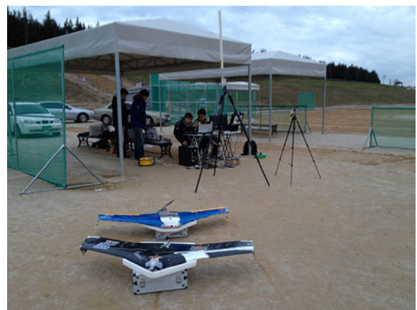
Fig. 7 Multi-agent testbed based on fixed-wing UAVs
