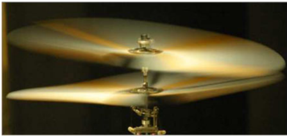
Fig. 15 Rotating coaxial rotor with lateral wind disturbances from the wind tunnel
