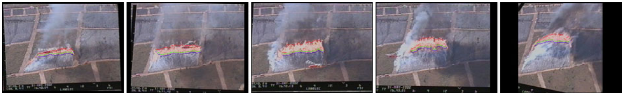
Fig. 13 Frames 3, 44, 77, 144 and 219 of the aerial sequence gathered during the fire experiment 520, after automatic stabilization. The extracted fire front contour is also shown
