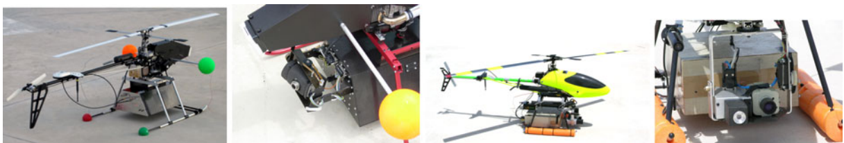
Fig. 3 The vehicles carry mainly IMUs and GPS for navigation. Also, visual and infrared cameras on pan and tilt units for environment perception have been used (see right photograph)
