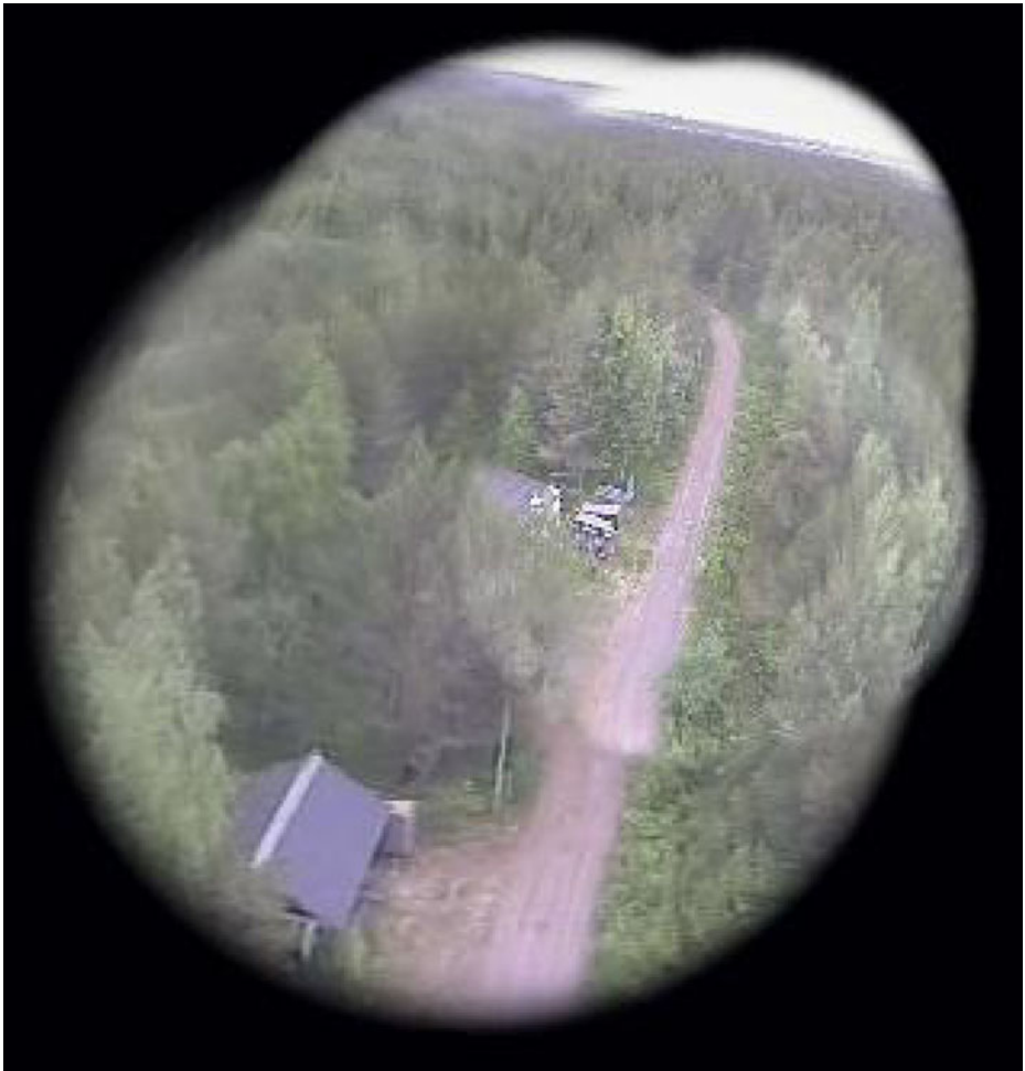
Fig. 8 An example of a photo map of the way of the UAV to the reconnaissance site (87 frames). Please note that there is a significant tilt of the camera and hence skew in the images. Though the algorithm is in theory not capable of registering under these conditions, the result is nevertheless quite usable of a rough orientation
