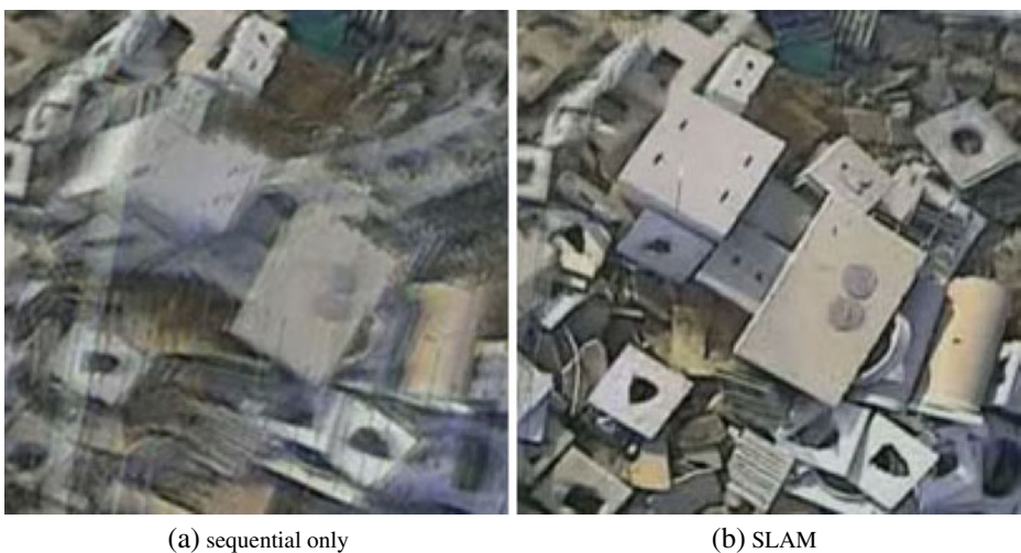
Fig. 15 A detail of the rubble pile map, once generated with sequential registration only ( left ) and once embedded in posegraph SLAM ( right )
