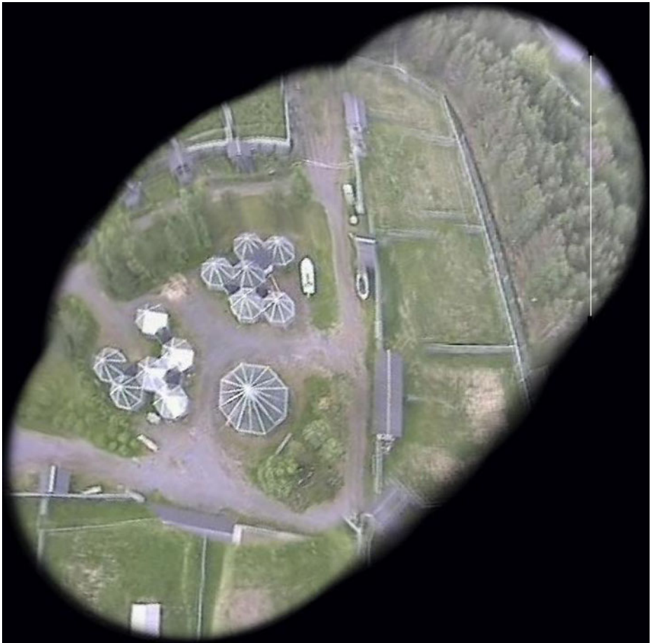
Fig. 12 A second example of a photo map of the camp generated from 784 video frames in real time
