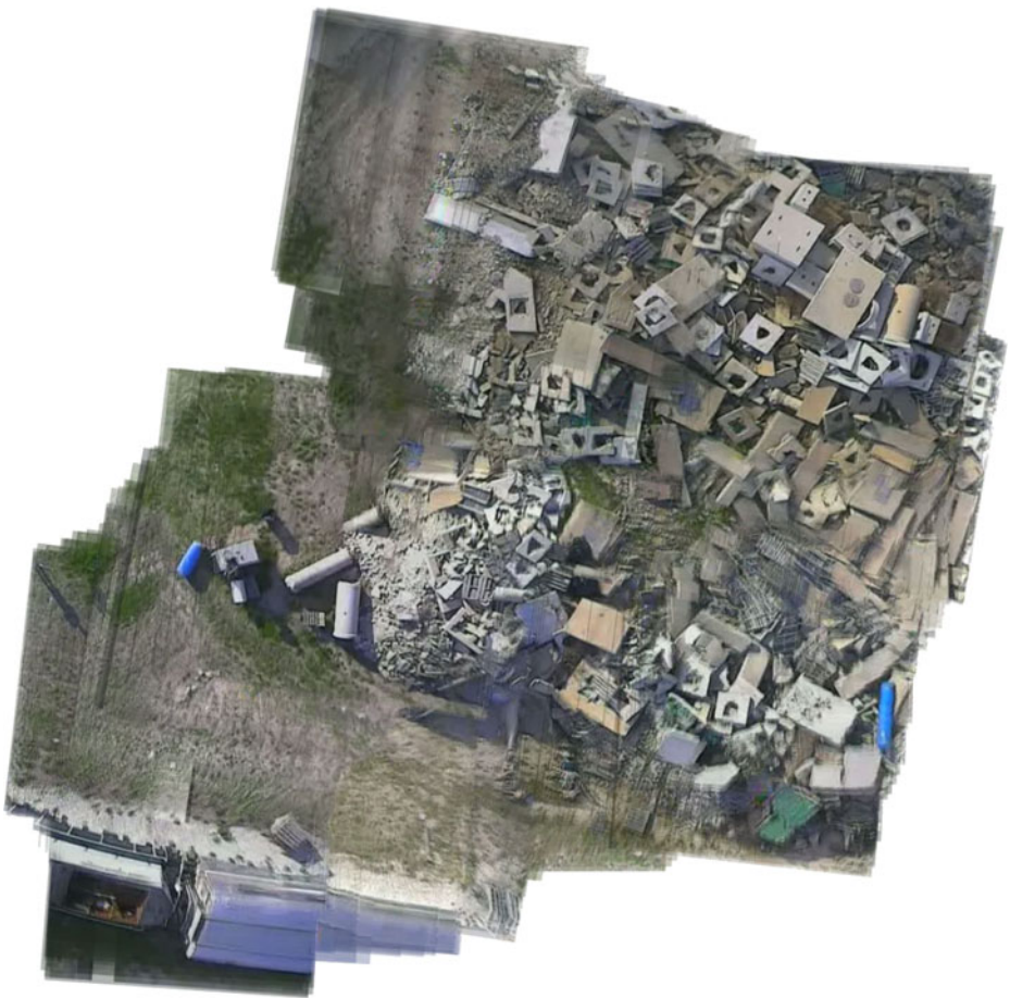
Fig. 13 A map of a rubble pile at Disaster City generated at RREE-2010 from 630 video frames via iFMI-SLAM
