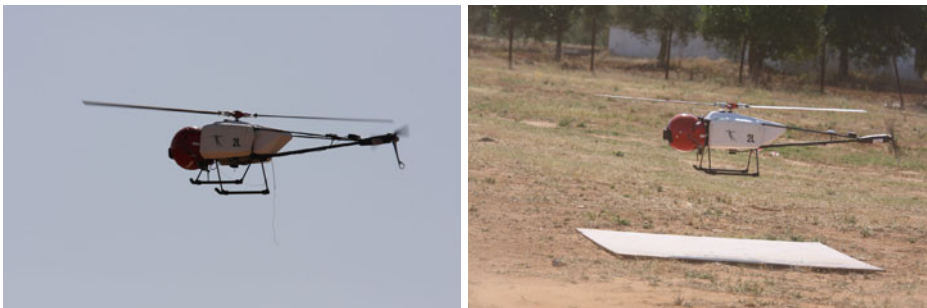
Fig. 5 The FC III E SARAH helicopter developed by the Flying-Cam (FC) company
