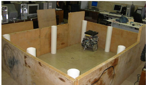
Fig. 10 Experimental setup with NAJI mobile robot: eight cylindrical landmarks are placed around wooden walls as point features
