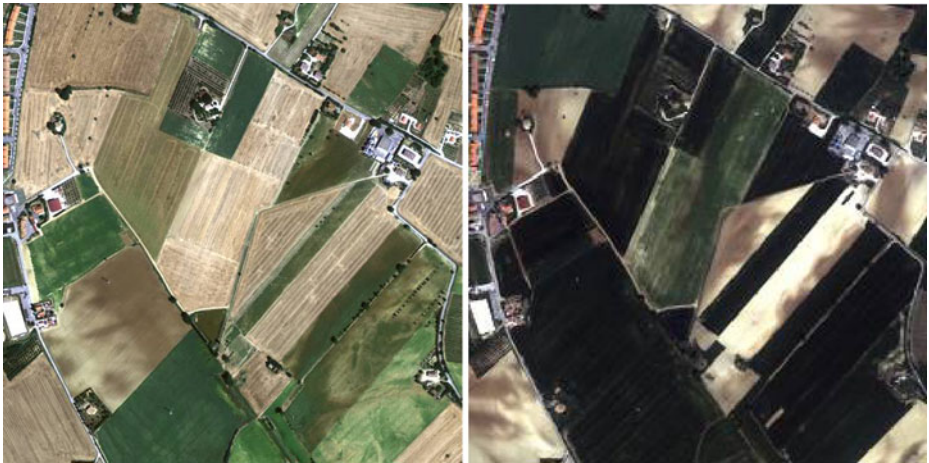
Fig. 2 Comparison of an aerial image and a satellite image of the same area. Significant differences in colours and boundaries of pieces of ground can be easily noted
