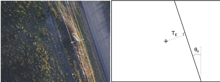
Fig. 1 Representation of linear features identified in the image plane through the use of track error, T_e , and observed line angle, \theta_o
