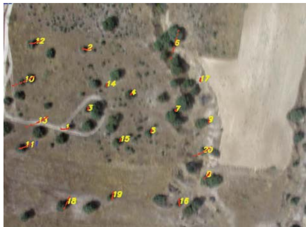
Fig. 13 Scene and tracked features during a non structured visual flight. Video sequence was taken by a manned helicopter traveling along a rectilinear trajectory for several hundred meters. The scene contains mainly non manmade features. Results are satisfactory although vibrations and image quality made the feature matching a difficult task
