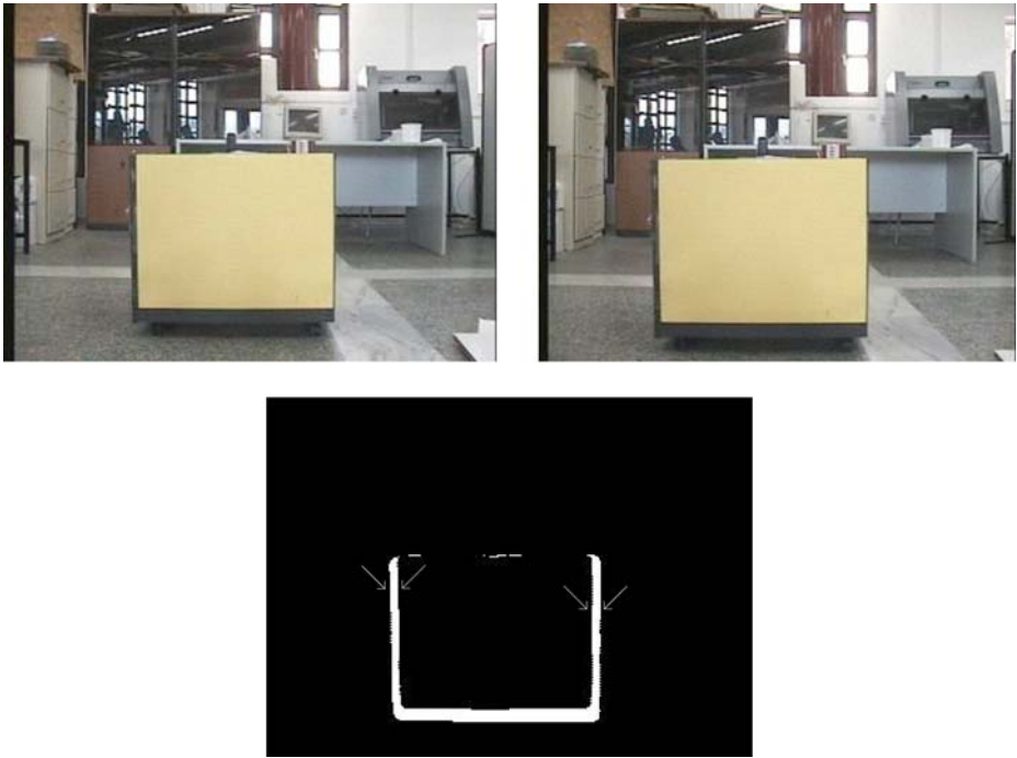
Fig. 24 Interesting point correspondence for the case of monocular vision system
