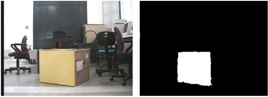
Fig. 25 Applying threshold technique in HSI color space
