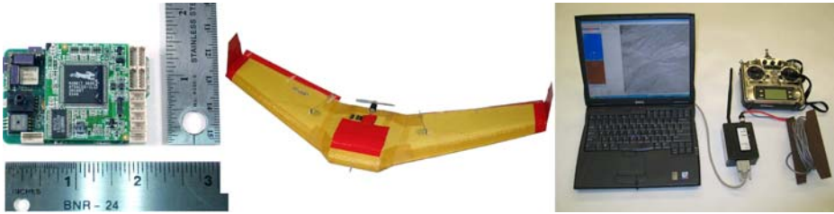
Figure 16 a Procerus' Kestrel autopilot. b MAV airframe. c Ground station components.
