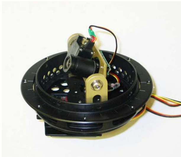
Figure 17 The gimbal and camera used for the results in the paper are shown unmounted from the MAV and without its protective dome.
