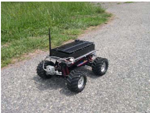
Figure 15. E-MAXX RC truck (UGV) with the on-board vision system.
