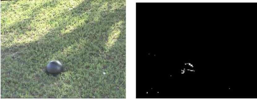
Figure 11. Fourth pair: Illustration of performance in different lighting conditions. Some pixels are misclassified due to the presence of shadow.
