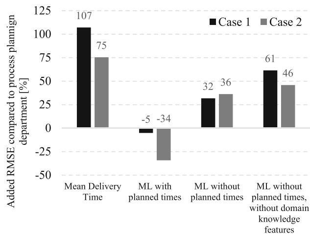
Fig. 10 Added error of approaches compared to prediction results of process planning department
