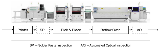
Fig. 7 Process chain for PCB assembly (picture by (Kitchenham et al., 2009))
