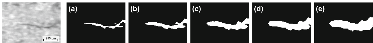
Fig. 4 Example of five different annotation types generated by dilating the original annotation shown in (a) with different morphological kernel sizes: b dilate=5, c dilate=9, d dilate=13 and e dilate=15
