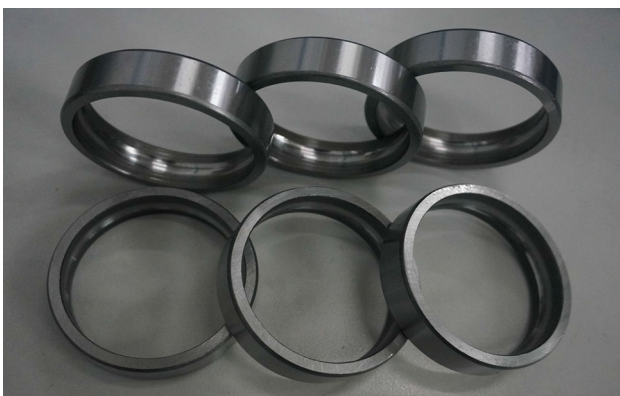
Fig. 4 Objective bearing rings to be machined
