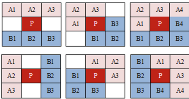
Fig. 4 CA mapping formats for selection of central cell
