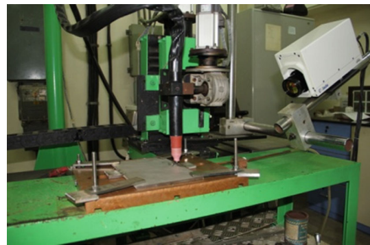
Fig. 2 GTAW setup with IR camera
