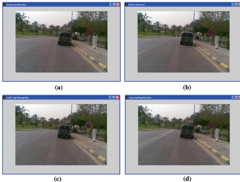
Fig. 21 On-road object recognition in the input frame. a Pedestrian detection, b vehicle detection, c road sign detection, d lane-marking detection
