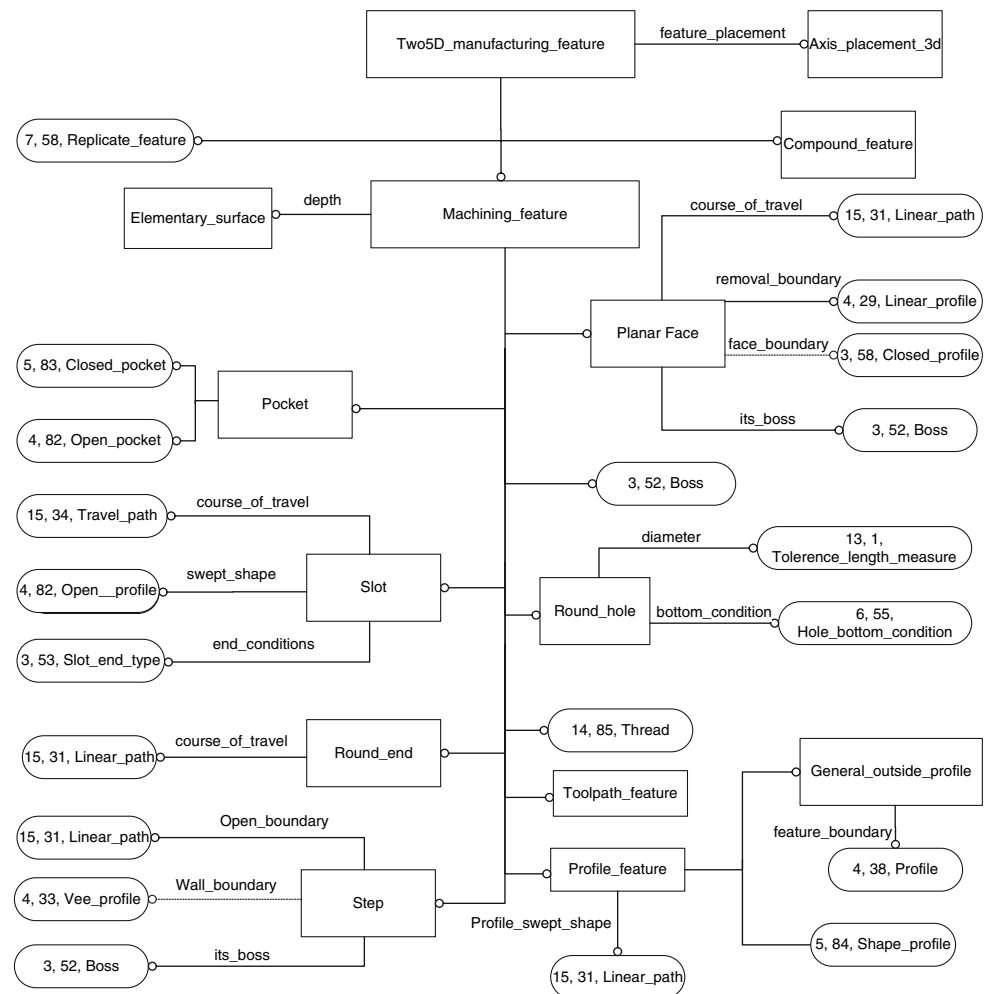
Fig. 3 EXPRESS-G schema of STEP-NC 2.5D manufacturing features (ISO 2003b)
