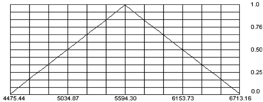
Fig. 5. Fuzzy cost for the problem with fuzzy flows represented by triangular membership function.
