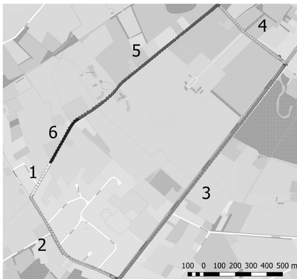
Fig. 9 An overview of the testing track with different colours indicating a different type of road. The total length of the circuit is about 5 kilometres. The track was traversed by three cars, that all traversed the track twice in 30 minutes. The numbered road types are respectively: (1) SMA type 1; (2) SMA type 2; (3) HMA; (4) Concrete plates; (5) Worn DAC (6) Very worn DAC
