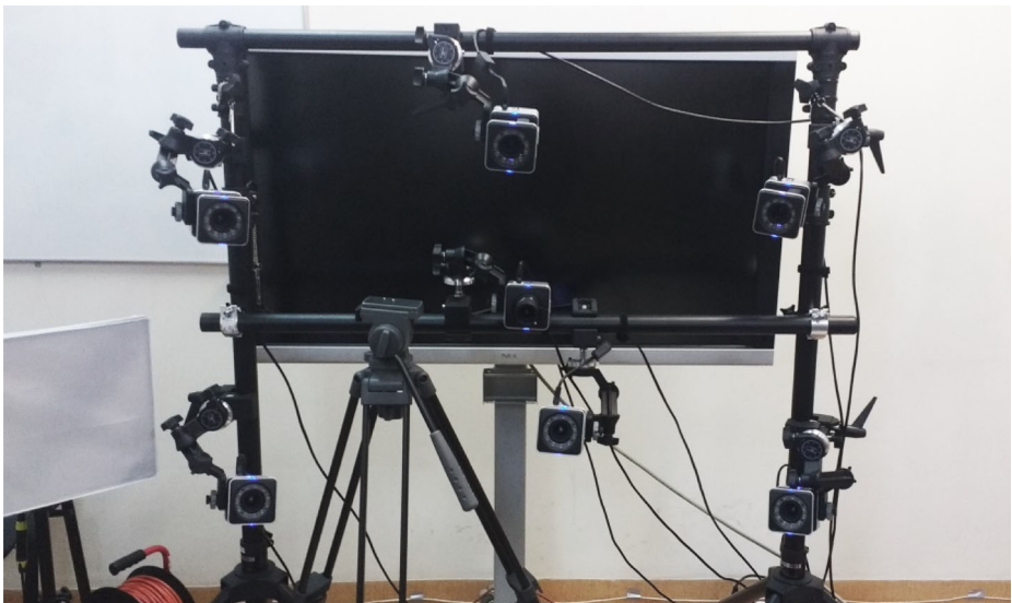
Fig. 4 A system of seven cameras to capture motion (Vicon 2018)
