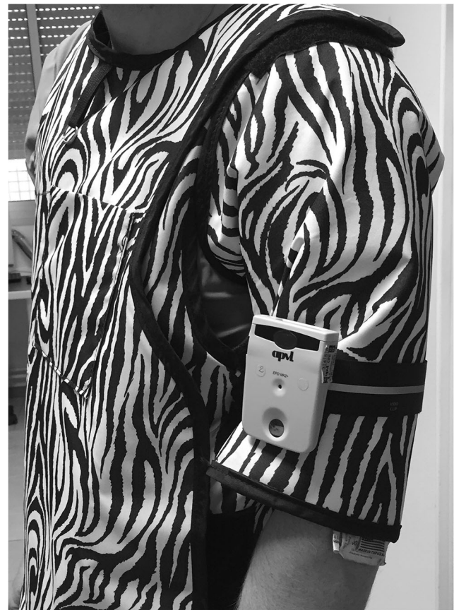
Fig. 1 Illustration of the personal electronic dosimeter located on the operator's left arm used to measure operator radiation exposure
