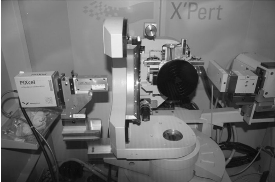
Fig. 3 The diffractometer-token used at the IJL
