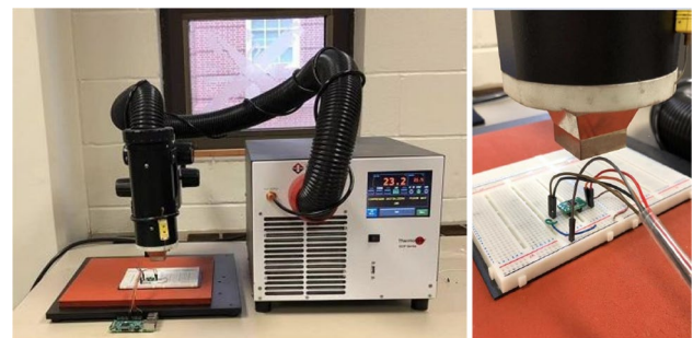
Fig. 9 Testing the SRAM at different temperatures with ThermoSpot direct contact probe system
