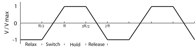
Fig. 2 Four-phased Landauer clocking
