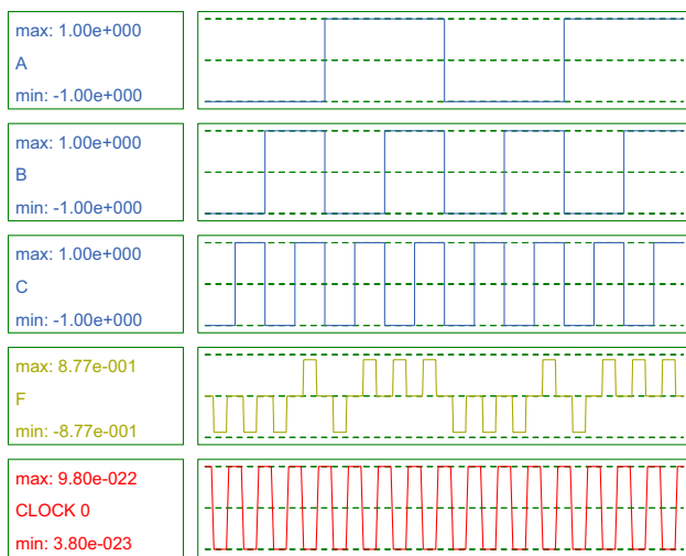
Fig. 5 Simulation of fault tolerant majority gate (ft-Maj)
