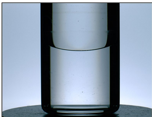
Fig. 7 Image of an 8 mL vial showing the organic (top) and aqueous (bottom) phases
