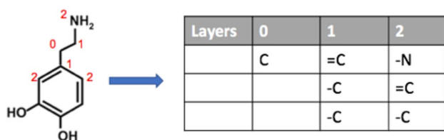
Fig. 1 Illustration of an atom environment. Molecule configuration with the heavy atoms being indexed based on its “layer” (left). 0-center atom; 1, 2-neighbor atoms that are 1 or 2 bonds away. Connectivity table of the atom environment (right)
