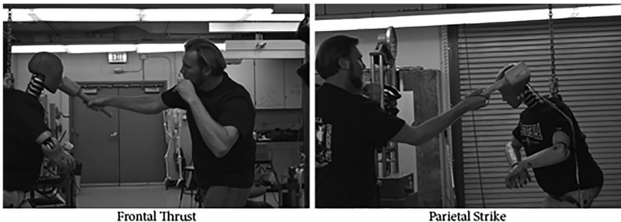
Fig. 4 Examples of ATD testing of frontal thrusts and parietal strikes. Photograph: Joseph Curran
