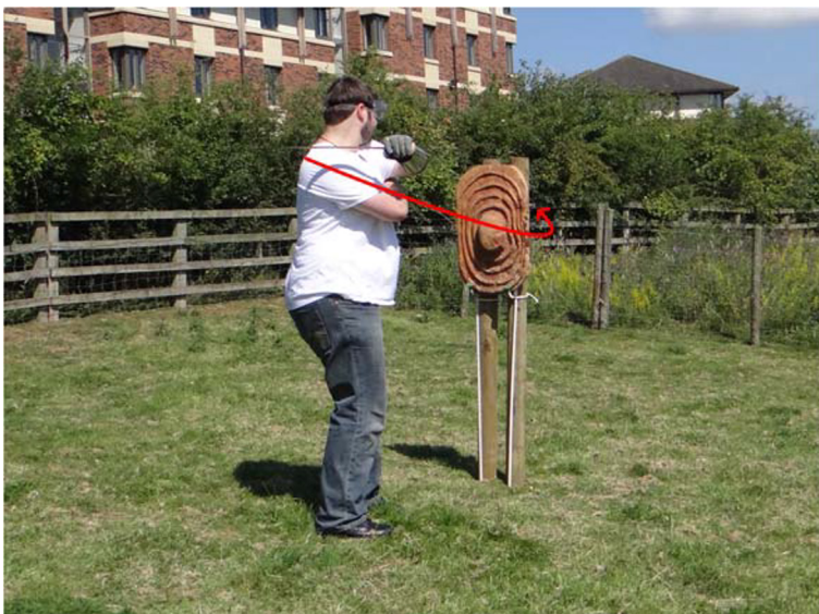
Fig. 14 Controlled weapon test 201b: glancing sword blow to the face of the wooden shield. This caused an irregular graze in the cutting edge
