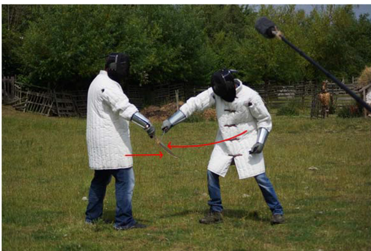
Fig. 20 Controlled weapon test 01k: leg strike vs dynamic flat parry. Note the defending sword (a Vollgriffschwert with wide leaf-shaped blade and narrow midrib) being bent by the incoming strike
