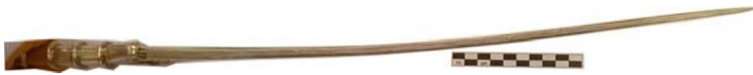
Fig. 17 Replica sword used in controlled weapon test 01k. Note the 10^\circ curvature from the original weapon axis
