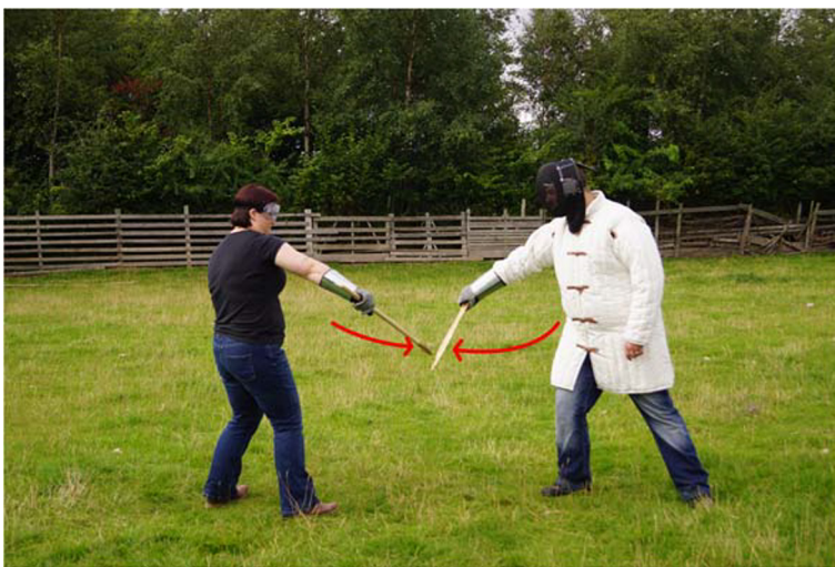
Fig. 6 Controlled weapon test 31e.4: long spearhead (on a short shaft) vs dynamic sword edge parry. This caused the formation of a wide-angled notch on the sword’s cutting edge
