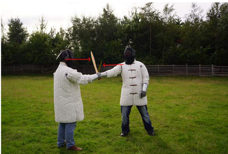
Fig. 16 Controlled weapon test 36a: shoulder strike vs static edge parry. This caused a rectangular indentation in the attacking sword
