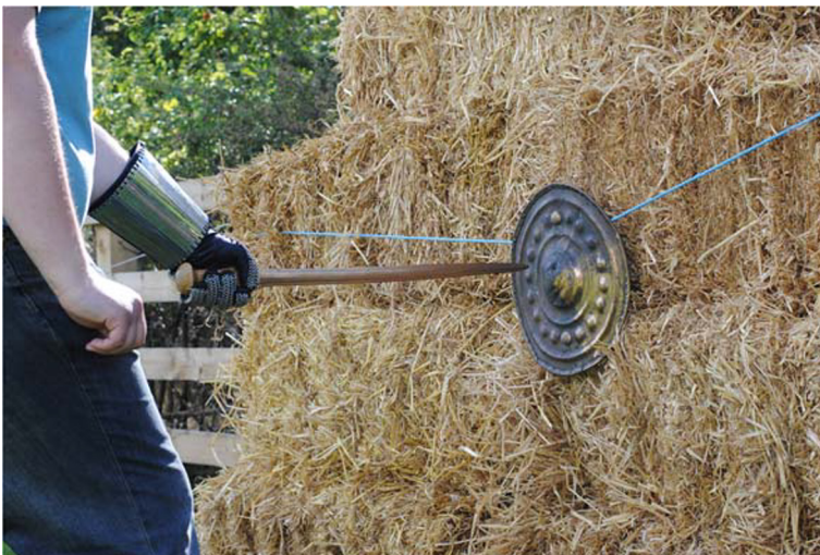
Fig. 12 Controlled weapon test 104a: static sword thrust to the face of the bronze shield mounted on hay bales
