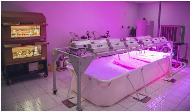
Fig. 1 Lumian AGS260 photobioreactor used for microalgae cultivation
