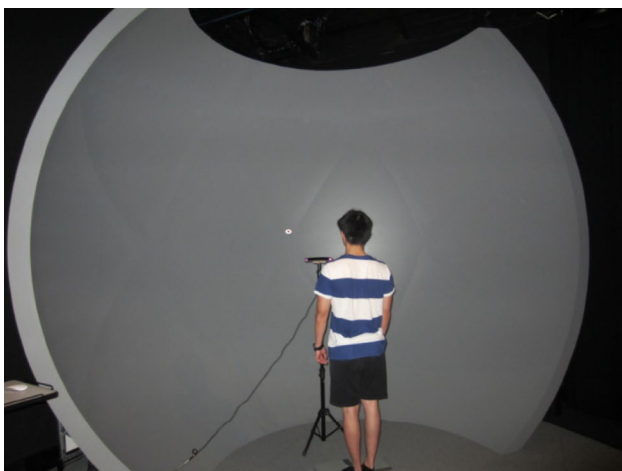
Fig. 1 Photo of a participant looking at the visual stimulus displayed on the half-dome concave screen while standing on the force platform. An eye tracker was placed in front of the participant
