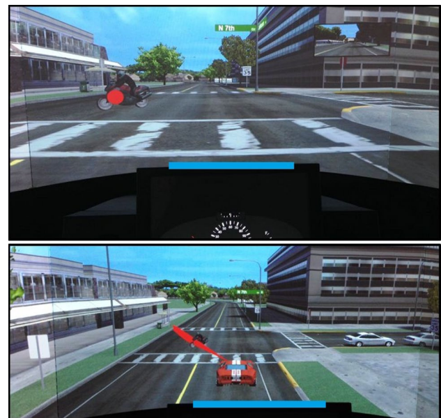
Fig. 2 Two types of eye-tracking feedback: driver view ( top red dot ) and aerial view ( bottom red line ). The thin horizontal bar above the dashboard represents the position of the integrated eye-tracker. (Color figure online)
