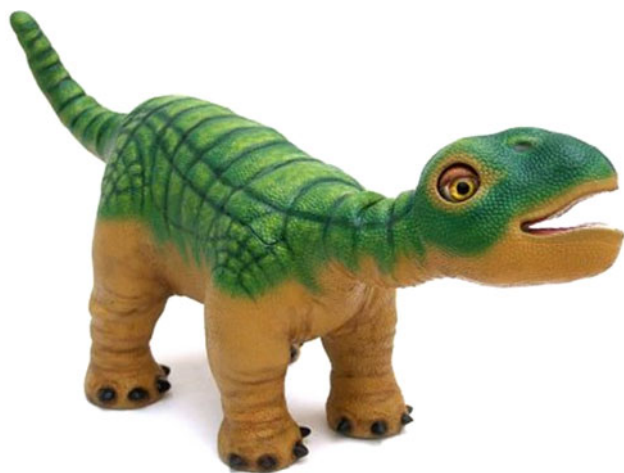
Fig. 1 The socially expressive robot Pleo. In the robot condition, participants interacted with Pleo, a small, commercially produced, toy dinosaur robot. Pleo is about 21 inches long, 6 inches wide, and 8 inches high, and was designed to express emotions and attention, using body movement and vocalizations that are easily recognizable by people, somewhat like a pet dog. For this study we customized Pleo's movements, synchronized with pseudo-verbal vocalizations, to express interest, disinterest, happiness, disappointment, agreement, and disagreement
