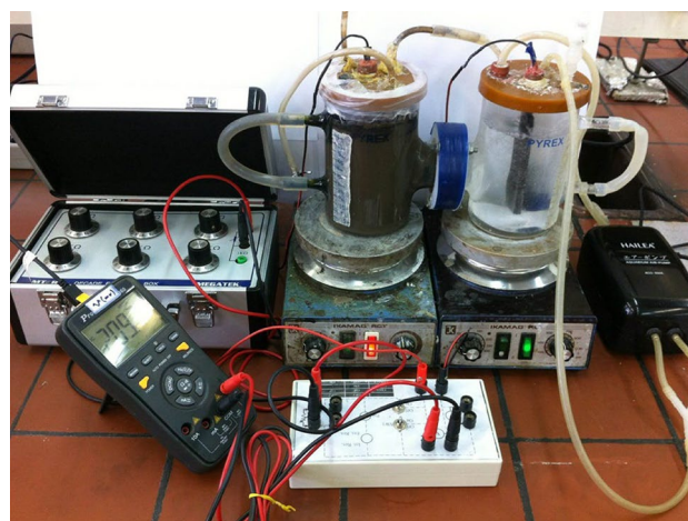
Fig. 1 Photograph of the laboratory-made two-chamber MFC reactor used in the present study
