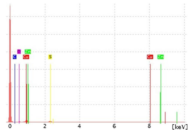
Fig. 10 EDS spectra of ZnS layers deposited at -1 , 0 V vs.SCE, on the copper substrate, at room temperature, for t=30 min
