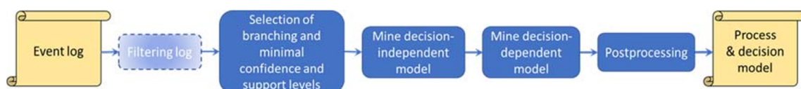
Fig. 5 The intermediate activities to go from the event log to an integrated process and decision model
