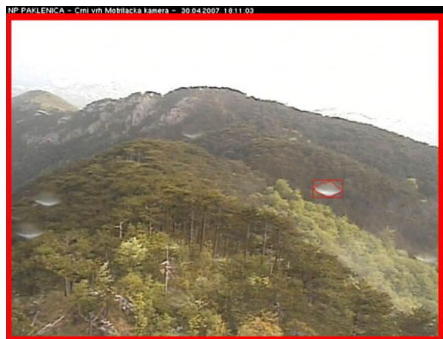
Fig. 10 False alarm caused by rain drop on the camera objective
