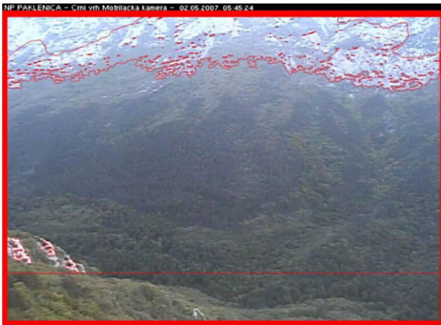
Fig. 11 False alarm triggered by abrupt change in environmental illumination (have large size vs. evolution time ratio)
