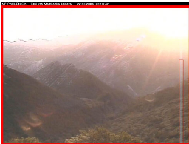
Fig. 12 False alarm triggered by sunlight effect on the camera objective (easily rejected using elongation factor)
