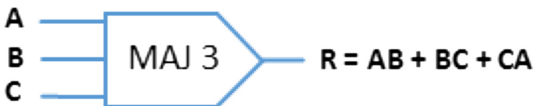
Fig. 10 Block diagram representation of output P of proposed SSG-QCA gate using majority voters
