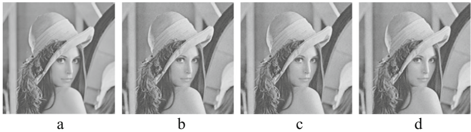
Fig. 10 Results of images with different compression ratios: a original image, b compression ratio 0.75, c compression ratio 0.5, d compression ratio 0.25
