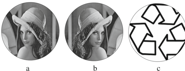
Fig. 8 Horizontal axisymmetry. a The stego image attacked by horizontal axisymmetry, (b) The stego image restored, (c) The watermark image extracted from (b)
