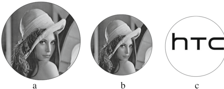
Fig. 10 Scaling attack. a The stego image attacked by scaling, (b) The stego image restored, (c) The watermark image extracted from (b)
