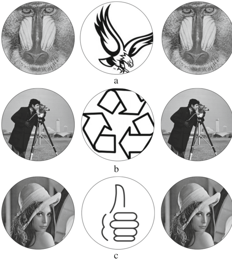
Fig. 13 In three groups of pictures, the left are the original carrier images, the middle are the watermark images, the right are the embedded carrier images
