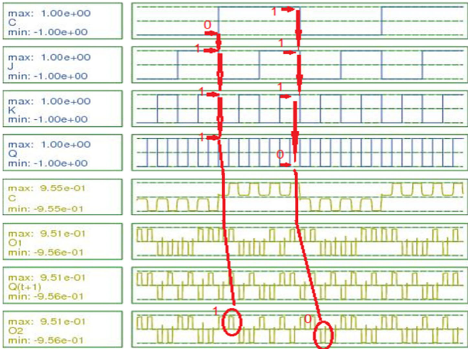
Fig. 13 Simulation result of proposed reversible JK flip-flop
