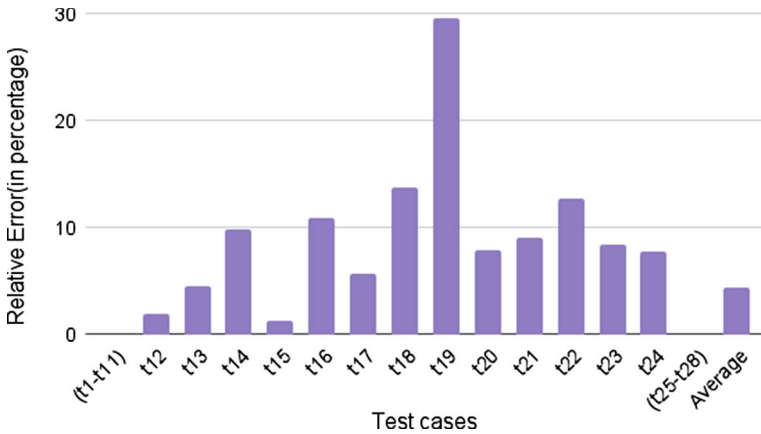
Fig. 22 Effect of memory access skipping on inaccuracy
