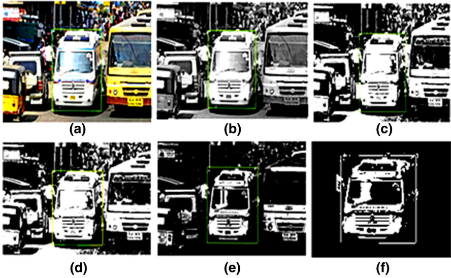
Fig. 6 a Emergency vehicle original image, b gray scale image, c threshold image, d edge detector, e erode image, f background image suppression
