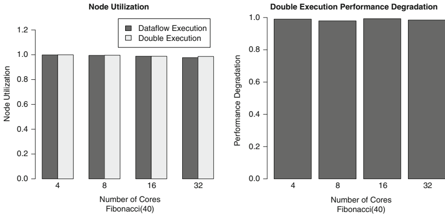
Fig. 9 Node utilization (left) and performance degradation for double execution of Fibonacci(40)
