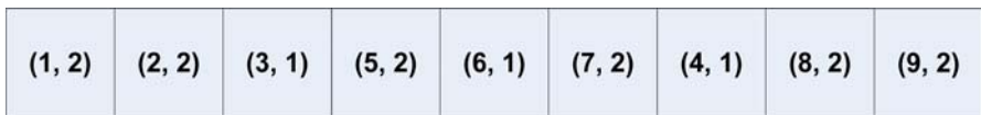
Fig. 3 The pair array of the chromosomes in Figs. 1b and 2. This pair is used to find the makespan and fitness for these chromosomes
