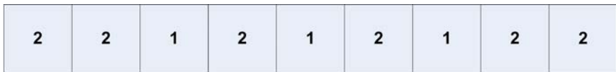
Fig. 2 An instance of chromosomes in PopP . In this example, it is considered that there are two processors to process the tasks of Fig. 1a. This figure shows the chromosome that is matched with chromosome in Fig. 1b
